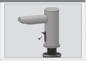
Connect the motor connector to its matching connector coming from the electronic unit. Please note that since the connector is water proof, some friction might apply.
